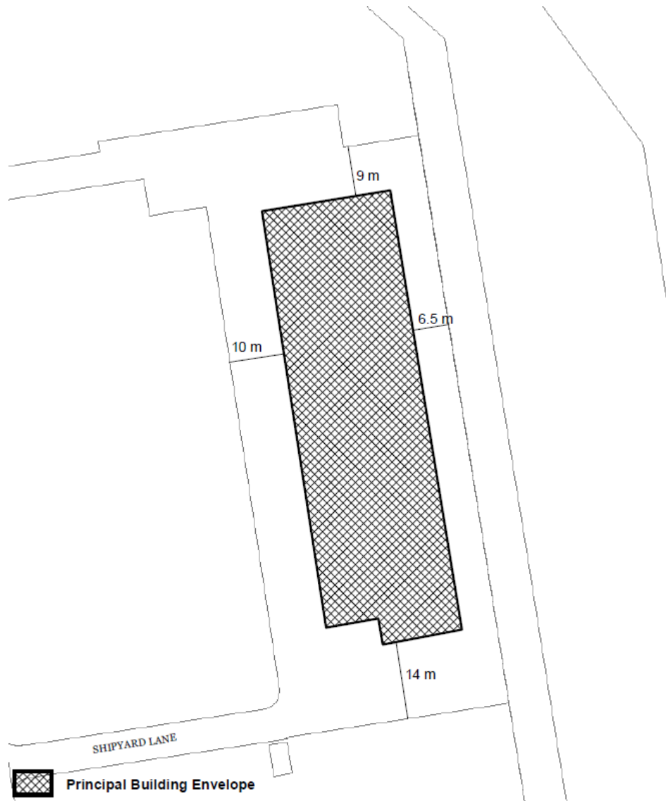
Illustration 7: R3-25 Zone requirements for building envelopes
