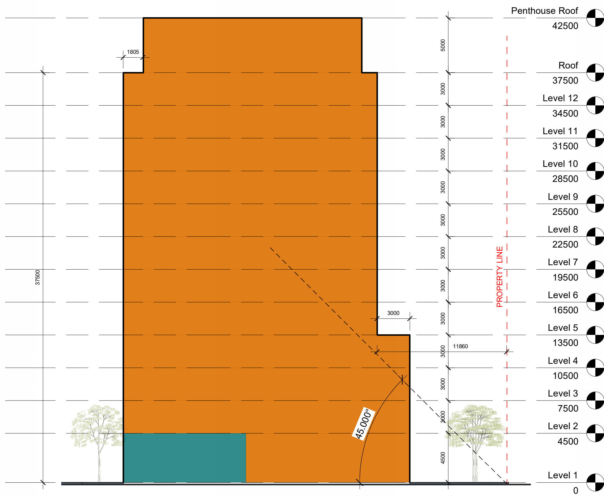
2 SOUTH-NORTH SECTION - MIXED USE BUILDING A104 1:200
