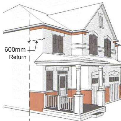
Detail of Material Return on Side Walls
