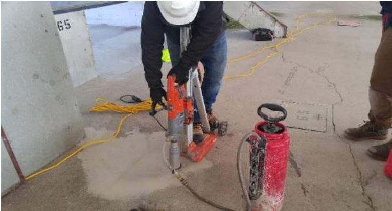
Figure 10 a, b: Slab Investigation (coring and scanning)
