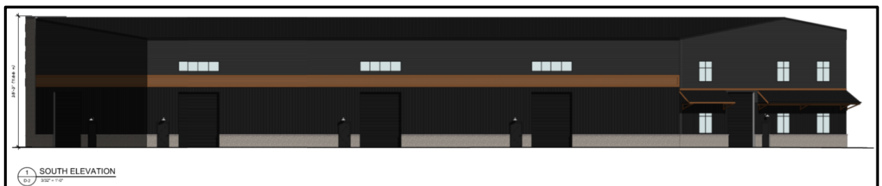
Figure 4: South elevation of Building 'B' showing roll-up loading doors
