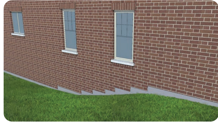
Foundation Wall at Sloping Grade
