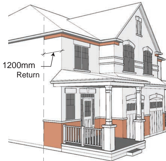
Detail of Material Return on Side Walls Examples of Architectural Detailing Requirements
