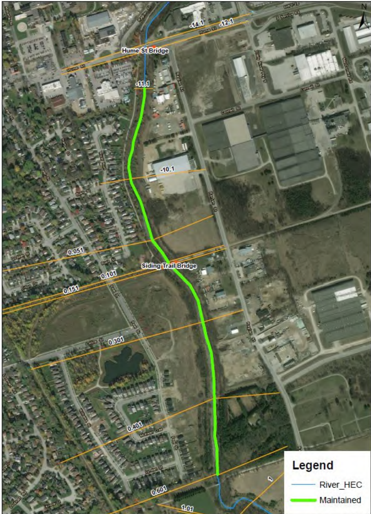
Figure 13: Maintained Section for Existing and Proposed Grading
