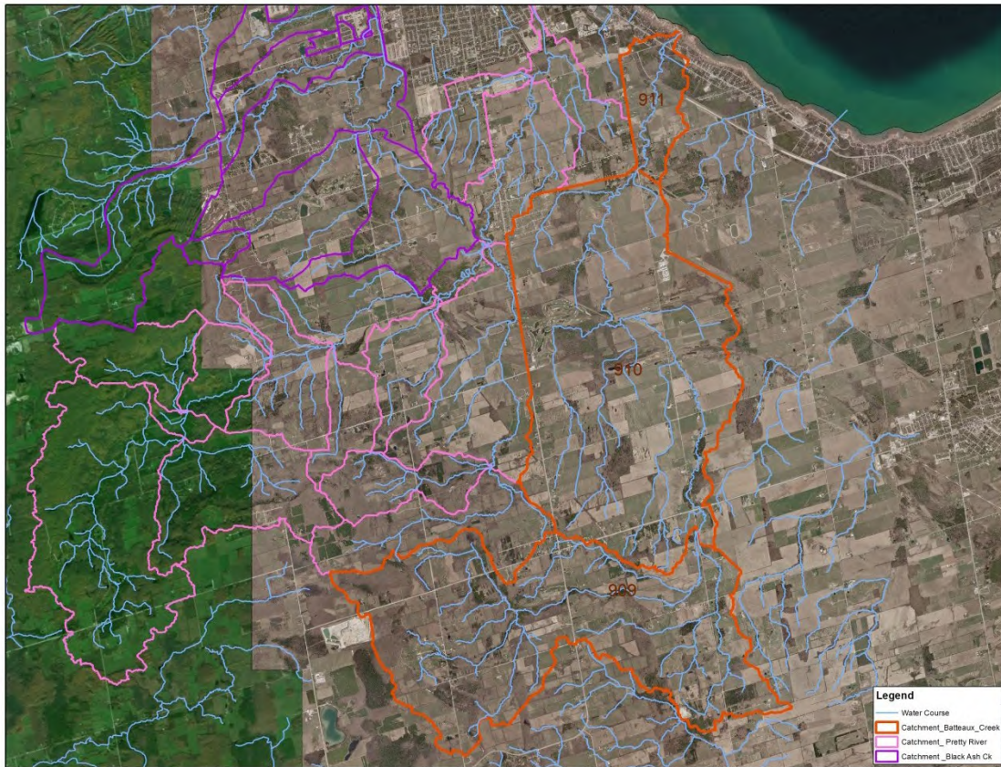
Figure 5- Batteaux Creek Updated Catchment Boundary
