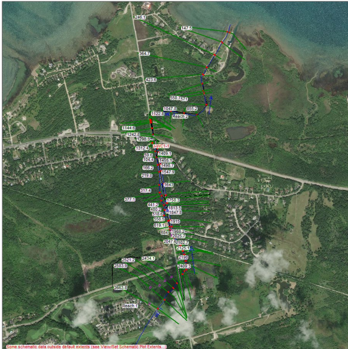
Figure 5-4 Townline Creek HEC-RAS Model Layout
