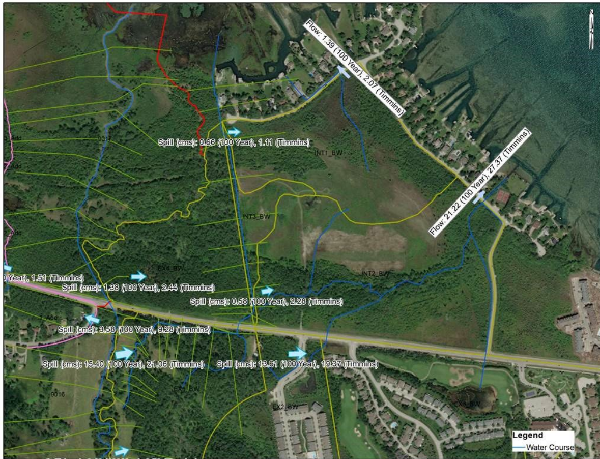
Figure 7-17 Spill Locations in Resort Areas
