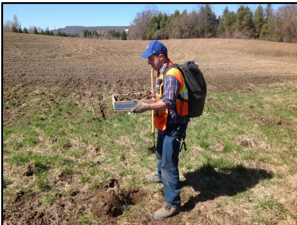
Image 14: Screening Soil through 6 mm Mesh (Photo Taken on May 1, 2015; Facing West)
