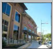
Plane breaks in the facade; fenestration changes; and, varied roof lines in this building could meet the standards of the UDM. Source: Peter French
