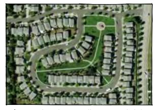
In this example, pedestrian walkways are included between rows of houses, to provide enhanced connectivity to the park at the north end of the block. Source: Google
