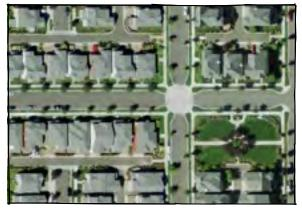
Pedestrian access and safety is improved in this location with: a. the use of curb extensions to reduce crossing distances and traffic speeds; b. sidewalks; and, c. a pedestrian scramble at the main park entrance. Source: Google
