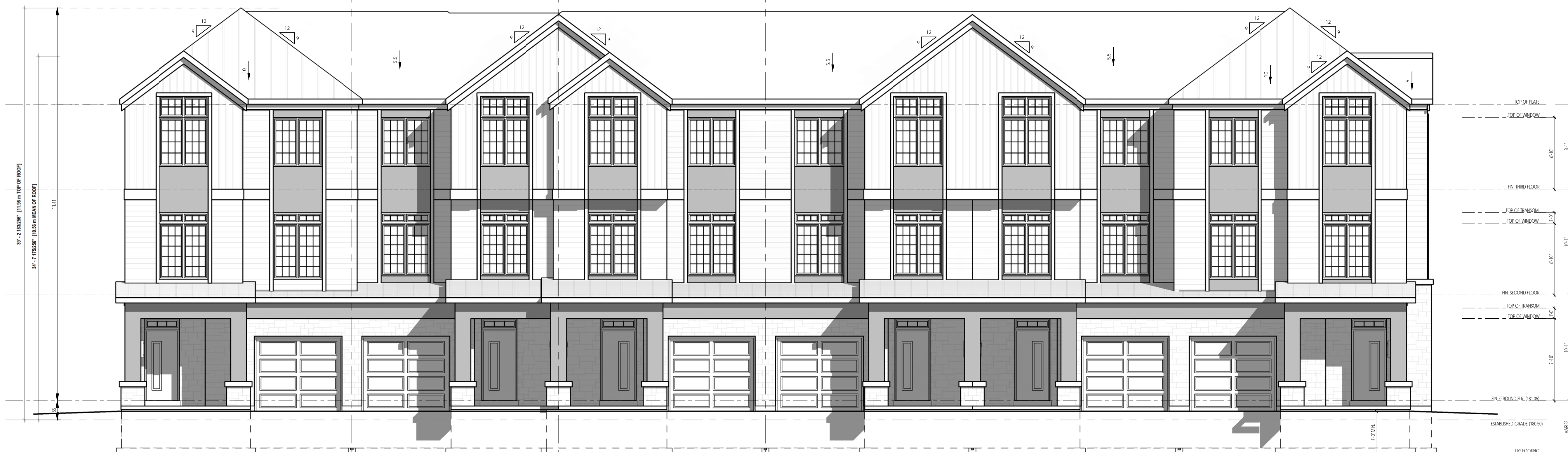
② BLOCK 1 - FRONT ELEVATION 3/16" = 1'-0" LOT 6 - UNIT 2002 BLOCK 1 LOT 5 - UNIT 2001 (REV.) BLOCK 1 LOT 4 - UNIT 2001 BLOCK 1 LOT 3 - UNIT 2001 (REV.) BLOCK 1 LOT 2 - UNIT 2001 BLOCK 1 LOT 1 - UNIT 2002 (LOT MOD.) (REV.) BLOCK 1
