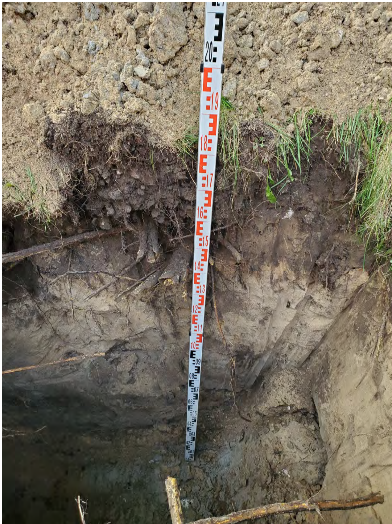
PHOTOGRAPH 1 Description: Detailed view of Test Pit #1 (depth measured).
