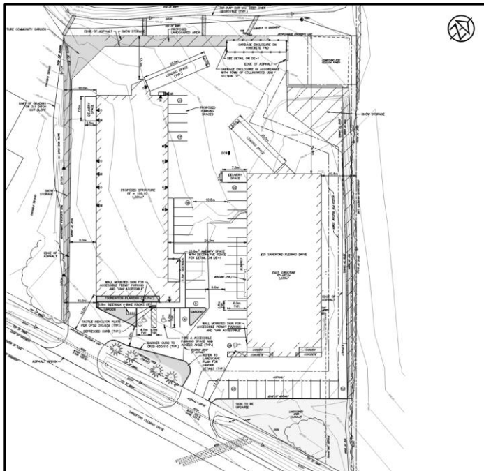
Figure 2 Proposed site plan with new building at left and existing on the right.
