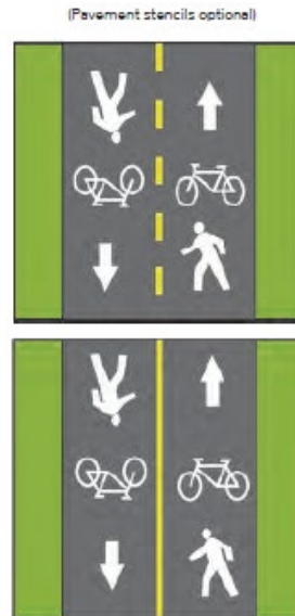
FIGURE 3.3: SAMPLE PAVEMENT MARKINGS FOR TWO-WAY SHARED USE PATH (Source: OTM Book 18, Figure 4.98, p. 120)
