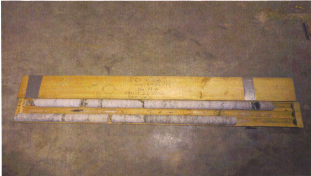
Figure # 3: Borehole 14-3 – Runs 1, 2 and 3
